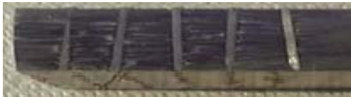
Laminate reinforced with z-pinning (z-fiber ® )
